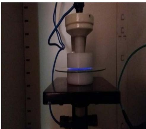
**Fig. 1. Locally design DBD plasma generator used in this study**
