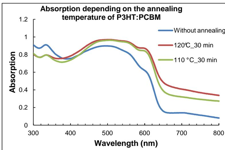
Fig. 5. Absorption depending of the thermal annealing as function of the wavelengths
