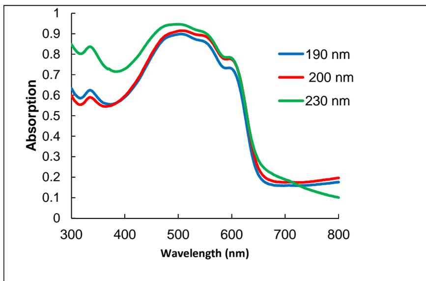
Fig. 4. Absorption of P3HT:PCBM as function of the thickness
