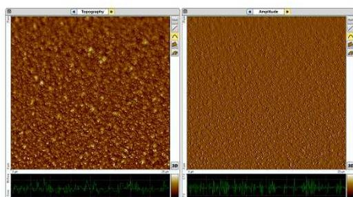
b- P3HT:PCBM annealed at 130°C during 30 min
