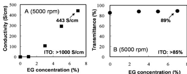
**Fig. 2. Plots of electrical conductivity (A) and visible-light transmittance (B) of the PEDOT/PSS thin films against concentration of (ethanol glycol) EG in the PEDOT/PSS dispersion used for the spin-coating [18]**
