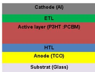
Fig. 3. Structure of the device realized
