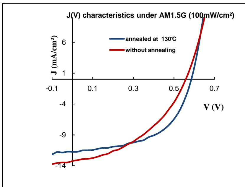
Fig. 6. Effect of the thermal annealing on the performance of the OPV
