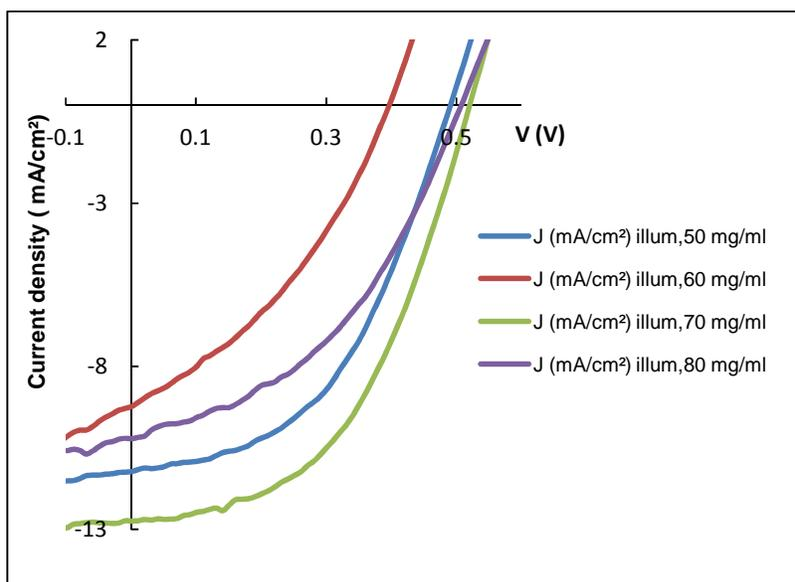
Fig. 7. Characteristic J (V) with different the concentration of the P3HT: PCBM blend
