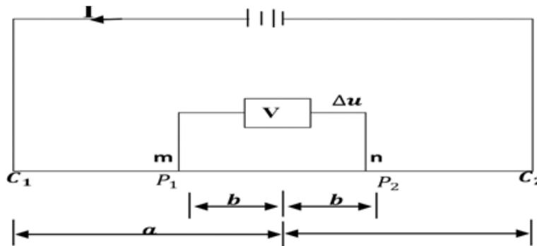
Fig. 3. Generalized Schlumberger electrode configuration resistivity measurement
