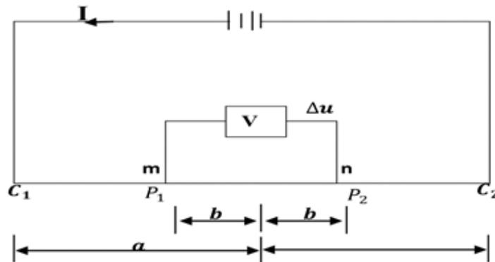
Fig. 2. General four (4) electrode configuration for resistivity measurement
