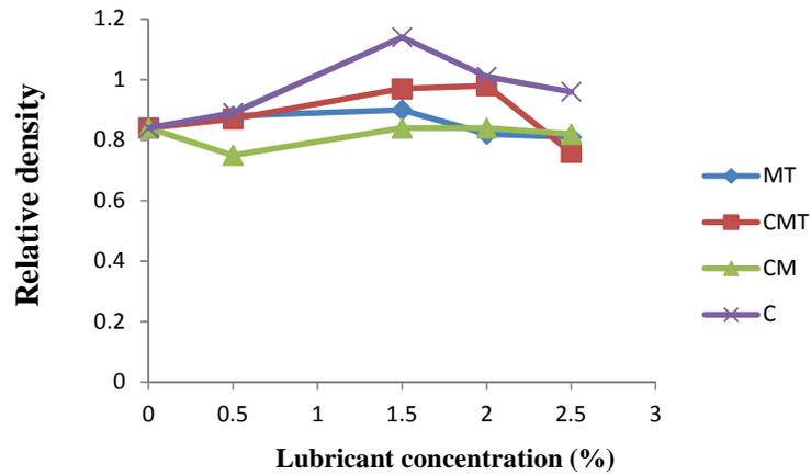
Fig. 1. Representative plot relative density versus lubricant concentration
