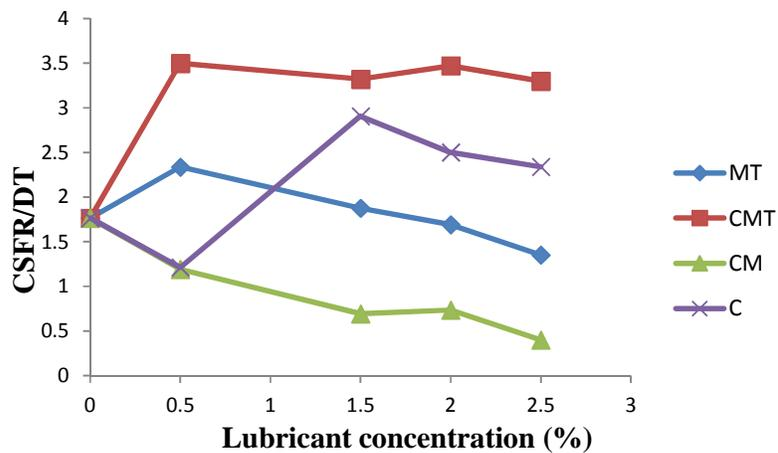
Fig. 5. Representative plot of CSFR/DT versus lubricant concentration
