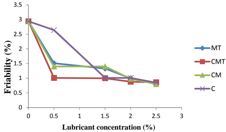
Fig. 3. Representative plot of % friability versus lubricant concentration
