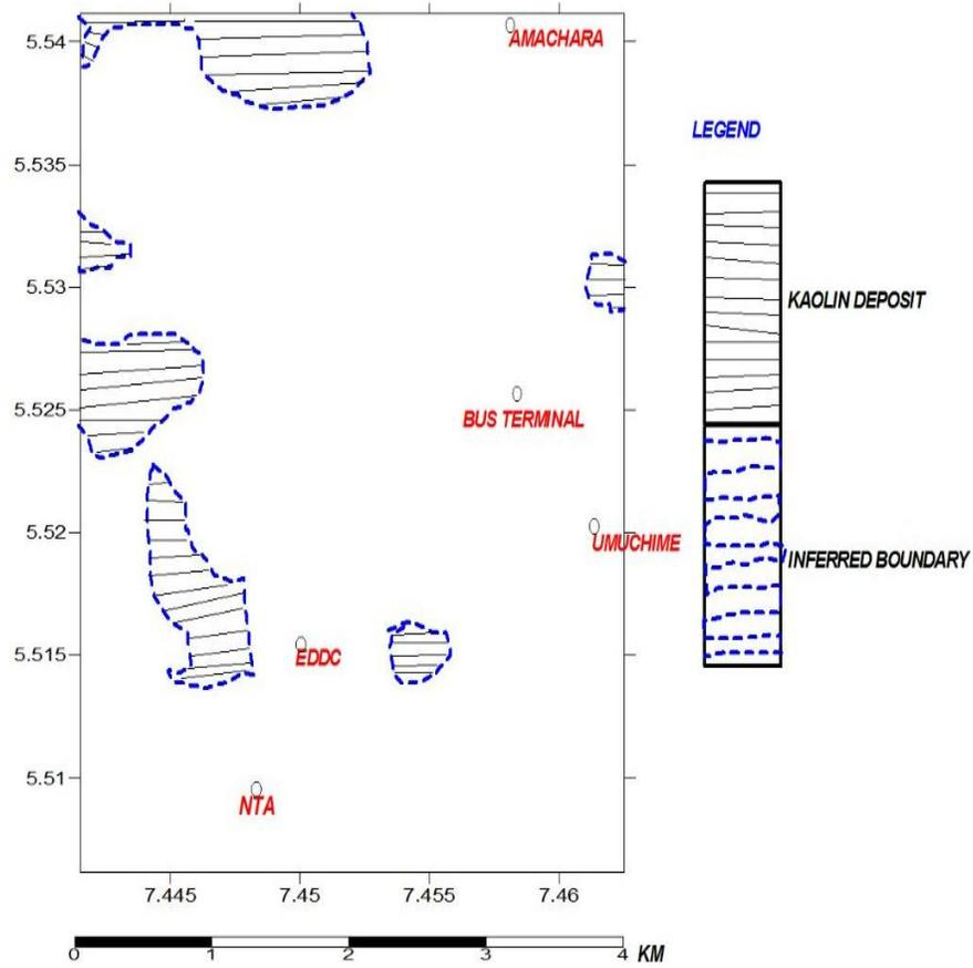
Fig. 7. Kaolin clay deposit inferred from sub-surface mapping
