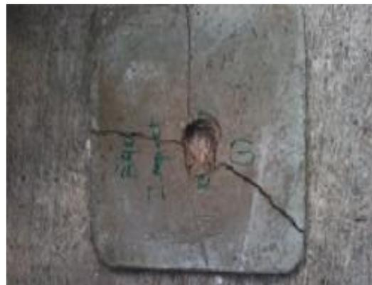
**Fig. 4. Specimen showing failure of B40 after impact-endurance test**
