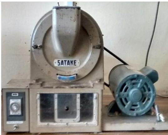
Fig. 3. Abrasive type polisher
