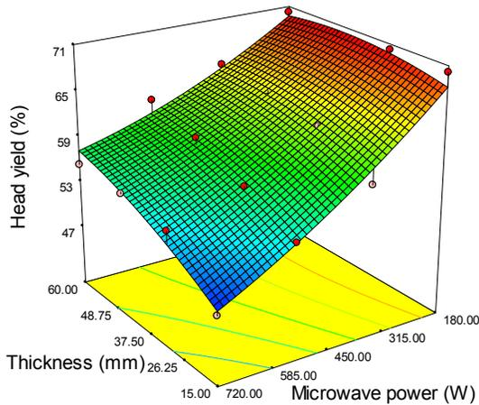
**Fig. 5. Effect of microwave power and bed thickness on head yield**
