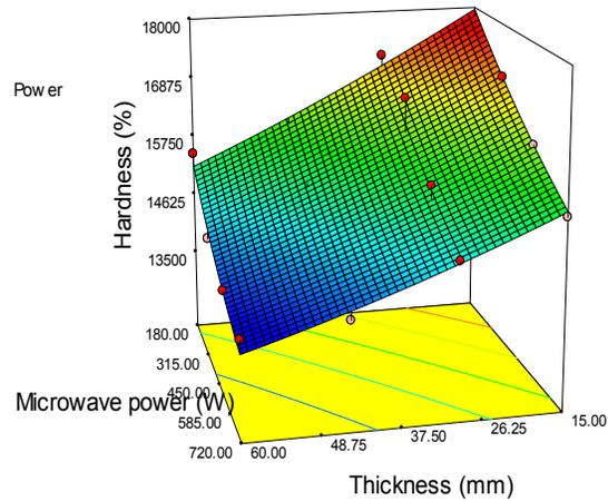
**Fig. 6. Effect of microwave power and bed thickness on hardness**
